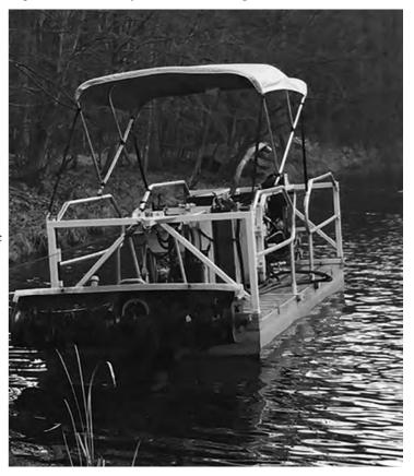
up and vacuum the mud and leaves and pump it across the road and into the large porous nylon pillows. The mud and vacuumed water goes in and the super fine mesh bag only lets the water leak out. The water soaks into the rocky forested gully behind the lot, leaving behind the slowly drying pillows of pure, rich, odor-free, organic soil.
